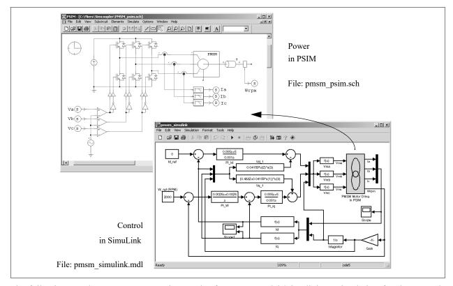
The following are the steps to set up SimCoupler for PSIM-Matlab/Simulink co-simulation for the example above.
