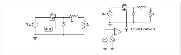
The circuit on the left uses a gating block, and the one on the right uses an on-off switch controller. The gating signal is determined by the comparator output.
