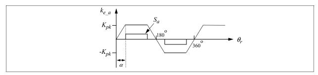
where  $K_{pk}$  is the peak trapezoidal value, in V/(rad./sec.), which is defined as:  $K_{pk} = \frac{V_{pk}/krpm}{2} \cdot \frac{1}{1000 \cdot 2\pi/60}$ . Given the values of Vpk/krpm and Vrms/krpm, the angle  $\alpha$  is determined automatically in the program.
