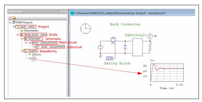
In this example, the project is the buck converter. It contains one study. The main circuit is "buck - main.psimsch", and the subcircuit is "buck - sub.psimsch". There are two simulation waveforms: I(S1.L1) and Vo.
