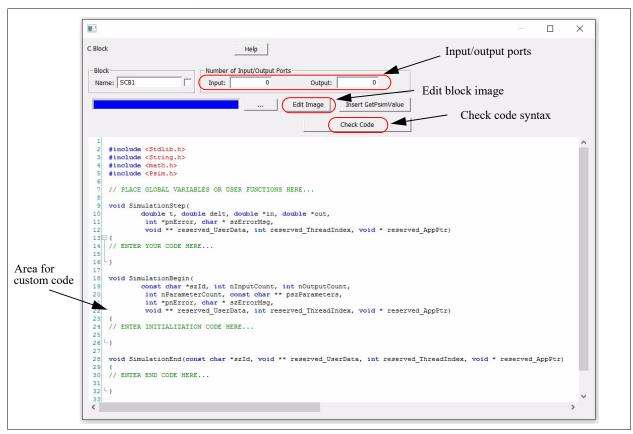
The number of input and output ports of the C block is defined in the *Number of Input/Output Ports* section. If the number of ports is changed, the image of the block in the schematic will change accordingly.
