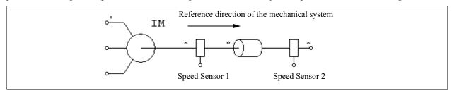
The torque sensor measures the torque difference between the dotted side of the sensor and the undotted side. To understand the physical meaning of the torque sensor measurement, we use the diagram below as an illustration.
