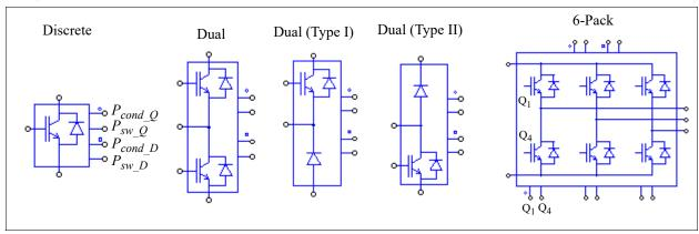
In the images, beside the IGBT and diode terminal nodes, there are four extra nodes from the top to the bottom (or from the left to the right on the top for the 6-pack package). They are the nodes for transistor conductor losses  $P_{cond}$  (the node with a circle), for transistor switching losses  $P_{sw}$ , for diode conductor losses  $P_{cond}$ . (the node with a square), and for diode switching losses  $P_{sw}$ , respectively.
