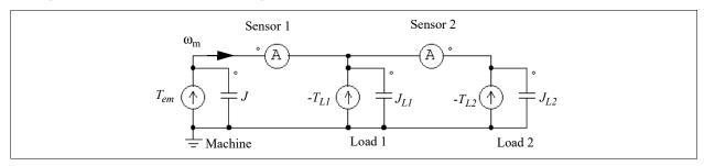
The node voltage in the circuit represents the mechanical speed  $\omega_m$ . The current probe on the left represents the reading of the Torque Sensor 1. Similarly, the current probe on the right represents the reading of the Torque Sensor 2. Note that the second current probe is from right to left since Sensor 2 is opposite to the reference direction of the mechanical system.
