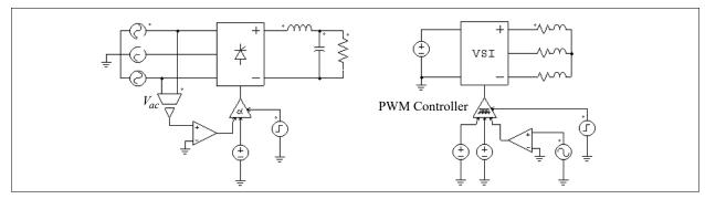
The thyristor circuit on the left uses an alpha controller. For a three-phase circuit, the zero-crossing of the voltage  $V_{ac}$  corresponds to the moment when the delay angle alpha is equal to zero. This signal is used to provide synchronization to the controller.
