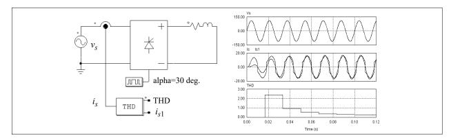
One of the THD block output is the input current fundamental component  $i_{s1}$ . By comparing the phase difference between the input voltage  $v_s$  and the current  $i_{s1}$ , one can calculate the input displacement power factor. This, together with the THD value, can be used to calculate the input power factor.
