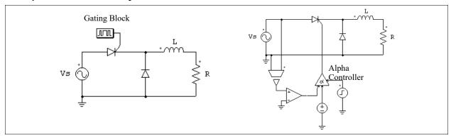
This circuit on the left uses a switching gating block. The switching gating pattern and the frequency are predefined, and remain unchanged throughout the simulation. The circuit on the right uses an alpha switch controller. The delay angle alpha, in deg., is specified through the dc source in the circuit.
