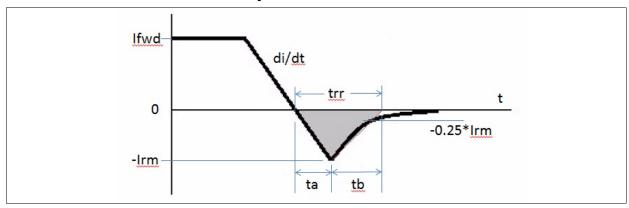
The reverse recovery time *trr* consists of two parts: *ta* and *tb*. During the period *ta*, the current increases from 0 to *-Irm*. Based on JEDEC (Joint Electron Device Engineering Council), *tb* is defined as the interval from the time of *-Irm* to the time when the straight line from *-Irm* through -0.25\**Irm* (in red in the diagram) intersects with the time axis.
