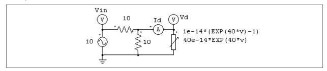
The nonlinear element (NONI) in the circuit above models a nonlinear diode. The diode current is expressed as a function of the voltage as:  $i = 10^{-14} * (e^{40*v}-1)$ . In PSIM, the specifications of the nonlinear element will be:
