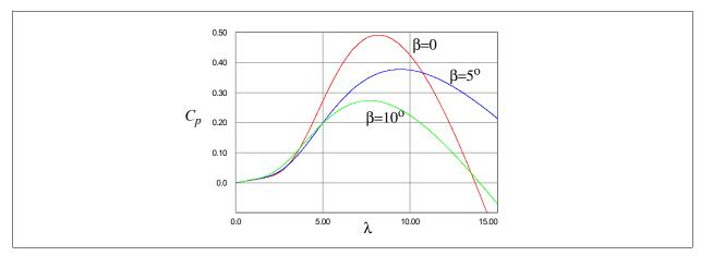
The figure shows that the power coefficient  $C_p$  reaches the maximum of 0.49 when the tip speed ratio  $\lambda$  is 8.18. We choose the values of  $C_p$  and  $\lambda$  at the maximum as the nominal values, i.e.,  $C_{p\_nom} = 0.49$ ,  $\lambda_{nom} = 8.18$ . One way to control the wind turbine, therefore, is to maintain the tip speed ratio at or close to the nominal value so that the power that the wind turbine generates is at the maximum.
