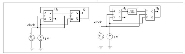
In the circuit on the left, the initial values of both  $Q_0$  and  $Q_1$  are assumed to be zero. At the clock rising edge,  $Q_0$  will change to 1. Without delay, the position of  $Q_1$ , which should remain at 0, will toggle to 1 at the same time.
