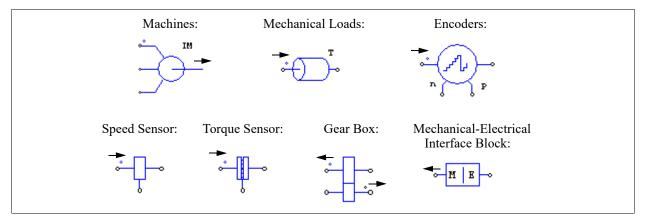
The reference direction of each element and the reference direction of the overall mechanical system determine how the element interacts with the mechanical system.
