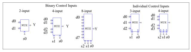
In the images, d0...d7 are the data inputs; and s0..s2 are the control inputs. The truth tables of the multiplexers are as follows.
