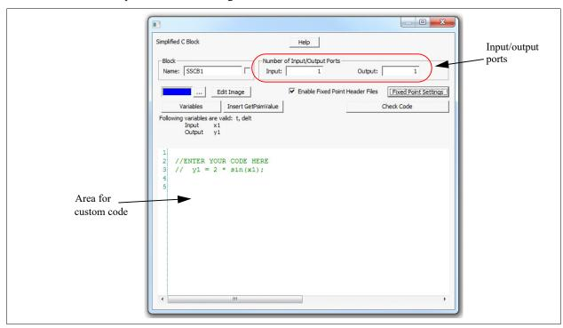
The number of input and output ports of the ports is defined in the *Number of Input/Output Ports* section. After the number of ports is changed, the image of the block in the schematic will change accordingly.
