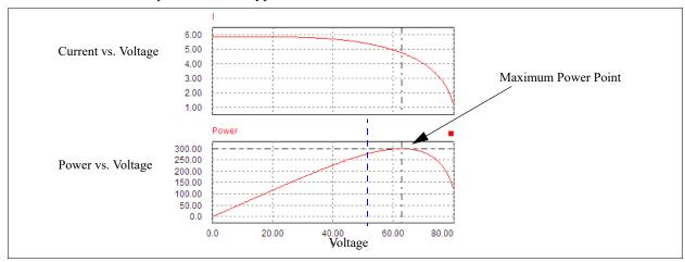
The curves show that the solar cell output power reaches the maximum at a specific voltage level. Many control
