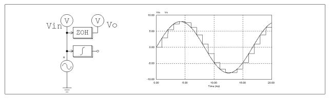
Note that in above circuit, a continuous-domain integrator is also connected to the input sine source. This makes it a mixed continuous-discrete circuit, and a simulation time step selected for the continuous circuit will be used. With this time step, the familiar staircase-like waveform can be observed at the zero-order hold output.
