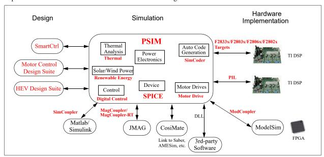
The PSIM simulation environment consists of the schematic program PSIM, two simulator engines (one PSIM engine and the other SPICE engine), and the waveform processing program SIMVIEW<sup>1</sup>. The simulation process is illustrated as follows.
