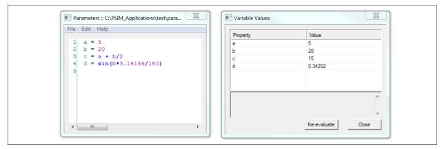
The function Show Values provides a very convenient way of checking the calculation.
