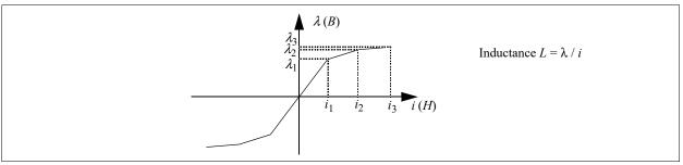
The inductance is defined as:  $L = \lambda / i$ , the ratio of  $\lambda$  vs. i at each point. The saturation characteristics are defined by a series of data points as:  $(i_1, L_1)$ ,  $(i_2, L_2)$ ,  $(i_3, L_3)$ , etc.
