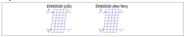
In the image, the nodes marked with the "+" and "-" signs are the positive and negative terminals. The node with the letter "S" refers to the light intensity input (in  $W/m^2$ ), and The node with the letter "T" refers to the ambient temperature input (in  $^{\circ}$ C).
