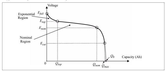
The capacity factor is roughly the ratio between  $Q_0$  (the capacity at 0V) and  $Q_{max}$ . It is a value close to 1, and it needs to be adjusted such that the battery voltage is equal to  $E_{cut}$  when SOC = 0.
