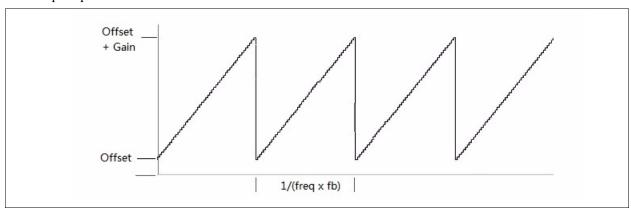
The output ramp frequency is the multiple of the input value and the base frequency fb. The output range is limited from -1 to +1. Therefore, the range of Offset and Gain must be limited as: Offset + Gain <= 1.
