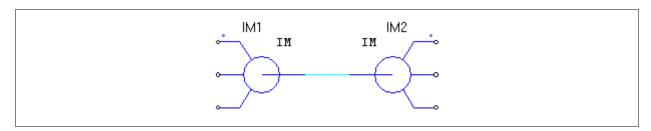
The system consists of two induction machines, IM1 and IM2, connected back-to-back. One operates as a motor, and the other as a generator. From the point of view of the first machine IM1, the mechanical equation can be written as:
