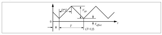
When the phase delay  $\theta$  is positive, the waveform is shifted to the right along the time axis.
