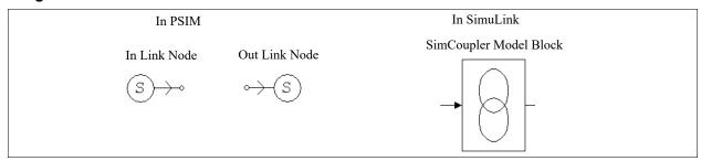
In PSIM, the In Link nodes receive values from Simulink, and the Out Link nodes send the values to Simulink. They are all control elements and can be used in the control circuit only. In Simulink, the SimCoupler model block is connected to the rest of the system through input/output ports.
