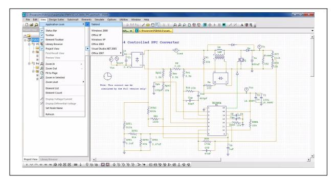
The Project View window provides an organized tree view of user's projects and their related files, as well as the simulation result graphs. Each PSIM circuit is treated as a project. The following content are displayed in stacking tiers in the project view:
