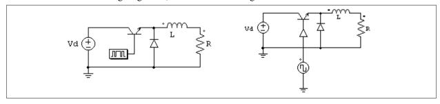
If the switch is controlled by a control circuit signal, as shown in the circuit on the right side, an on-off switch controller must be used at the gate node.
