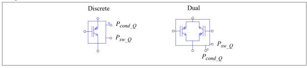
In the images, beside the IGBT terminal nodes, there are two extra nodes. They are the nodes for transistor conductor losses  $P_{cond\ O}$  (the node with a circle), and transistor switching losses  $P_{sw\ O}$ .
