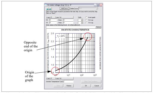
• In this step, the border of the graph area is defined by first left clicking at the origin of the graph (usually the lower left corner), then left clicking again at the opposite corner of the origin (usually the upper right cor-
