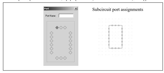
The diamonds on the four sides represent the connection nodes and the positions of the subcircuit. They correspond to the connection nodes of the subcircuit block on the right. There are no diamonds at the four corners since connections to the corners are not permitted.
