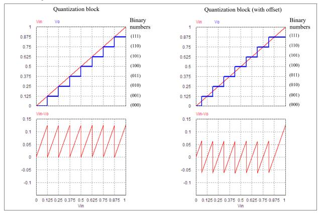
As shown from the waveforms on the left, the quantization error of the quantization block is from 0 to 1 LSB (least significant bit), or  $1/2^3$  (or 0.125).
