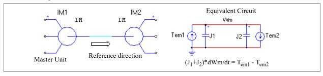
Similarly, if we define the machine IM2 as the master unit, the reference direction of the overall mechanical system will be from right to left, as shown below. Based on this direction, the machine IM1 will be opposite to the reference direction, and the machine IM2 will be along the reference direction. This leads to the equivalent circuit of the mechanical system as shown on the right.
