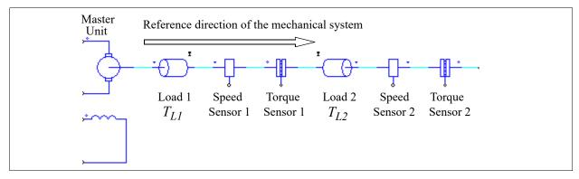
In this mechanical system, the machine on the left is the master unit. The reference direction of the mechanical system is from left to the right along the mechanical shaft. Comparing this direction with the reference direction of each element, Load 1, Speed Sensor 1, and Torque Sensor 1, will be along the reference direction, and Load 2, Speed Sensor 2, and Torque Sensor 2 will be opposite to the reference direction of the mechanical system.
