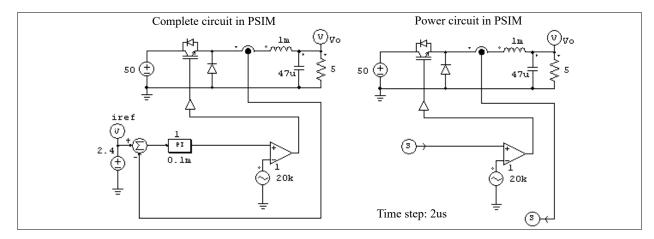
There are different ways of setting up Simulink to perform co-simulation. The recommend approach is to set the Solve Type to **Fixed-step** and define the **Fixed step size** to be the same or close to PSIM's time step. The figure below shows this option.
