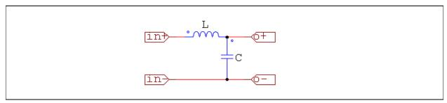
In this case, the inductance and capacitance values will be defined through the interface, and need to appear in the property window of the new LC filter element. Therefore, the parameter value for the inductance needs to be defined as a variable, in this case, L, and the value for the capacitance as C.
