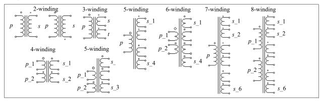
In the images, p refers to primary, s refers to secondary, and t refers to tertiary. The winding with the largest dot is the primary winding or first primary winding. For the multiple winding transformers, the sequence of the windings is from the top to the bottom. For the transformers with 2 or 3 windings, the attributes are as follows.
