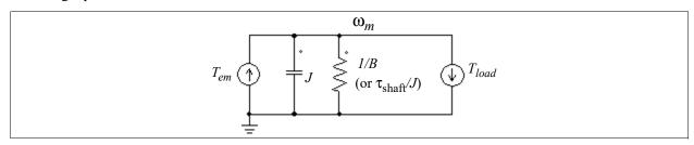
This circuit shows that the shaft time constant  $\tau_{\text{shaft}}$  is equal to the RC time constant of the resistor 1/B and the capacitor J. Therefore, the shaft time constant can be measured by the following test:
