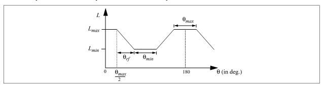
The rotor angle is defined such that, when the stator and the rotor teeth are completely aligned,  $\theta = 0$ . The value of the inductance can be in either rising stage, flat-top stage, falling stage, or flat-bottom stage.
