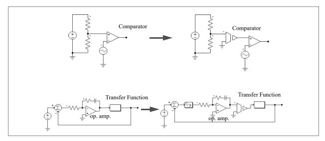
It should be noted that, in PSIM, the power circuit and the control circuit are solved separately. There is one time step delay between the power and the control circuit solutions.
