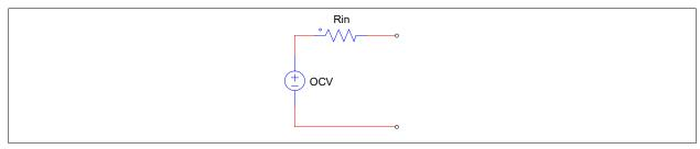
For the internal resistance Rin, two tables can be defined: one during the discharge process, and another during the charge process.
