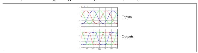
The fundamental component of the output is 1.155 times the value of the input.
