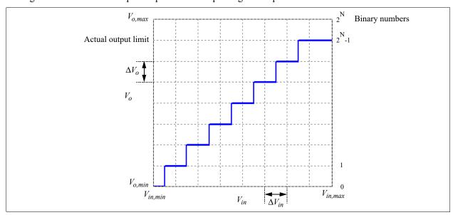
The number of bits determines the quantization resolution. The input range,  $V_{in,max}$  -  $V_{in,min}$ , is divided into  $2^{\rm N}$
