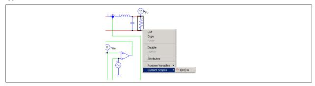
If the element has multiple current flags, under the *Current Scopes* menu, there will be multiply branch currents, one corresponding to each current flag.
