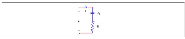
The mmf, in the form of a voltage source, applies across the capacitor (the capacitance has the value of the inductance factor  $A_L$ ) and the resistor R. For the element  $Air\ Gap$ , the inductance factor can be calculated from the air gap length and the cross section area as:
