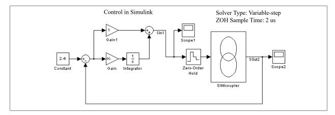
Therefore, Simulink must be set up to have the Solver Type as **Fixed-step** with the time step the same or close to the PSIM time step, or if the Solver Type is **Variable-step**, a zero-order-hold must be used with the sample time the same or close to PSIM time step
