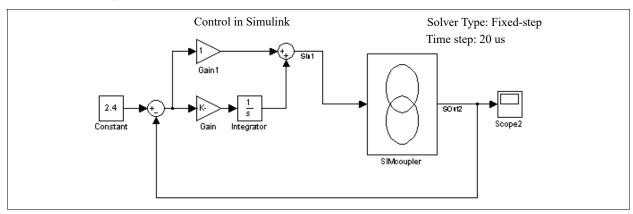
It is recommended that Simulink use the same time step as PSIM, although we have found that, even if the Simulink time step is slightly larger than PSIM time step, satisfactory results are obtained. In this case, for example, the time step is set to 20 us, 10 times larger than the PSIM time step.
