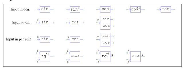
If the input of a block has the letter "r", it is in radian. If the input has the letter "u", it is in per unit. Otherwise it is in deg.
