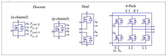
In the images, beside the MOSFET and diode terminal nodes, there are four extra nodes from the top to the bottom (or from the left to the right on the top for the 6-pack package). They are the node for transistor conductor losses  $P_{cond\_Q}$  (the node with a circle), for transistor switching losses  $P_{sw\_Q}$ , for diode conductor losses  $P_{cond\_D}$  (the node with a square), and for diode switching losses  $P_{sw\_D}$ , respectively.
