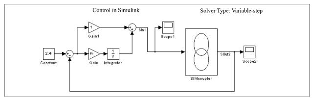
When the Simulink Solver type is set to **Variable-step**, in order to obtain correct results, a zero-order-hold must be placed at the input of the SimCoupler model block. Moreover, the zero-order-hold sample time must be the same or close to PSIM time step. The figure below shows the configuration.
