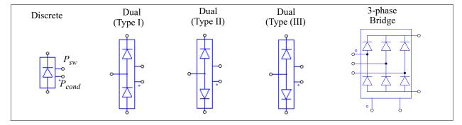
In the images, beside the diode anode and cathode terminals, there are two extra nodes. The node with a dot is for the diode conduction losses  $P_{cond}$ , and the node without a dot is for the diode switching losses  $P_{sw}$ .
