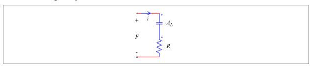
The mmf, in the form of a voltage source, applies across the capacitor (the capacitance is  $A_L$ ) and the resistor R. Let the current flowing through this branch be i, and the rms value be  $I_{rms}$ , the relationship between the losses due to the leakage flux and the resistance R is:
