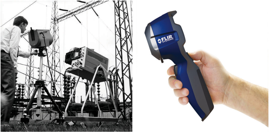
Figure 19.2 LEFT: Thermovision® Model 661 from 1969. The camera weighed approximately 25 kg (55 lb.), the oscilloscope 20 kg (44 lb.), and the tripod 15 kg (33 lb.). The operator also needed a 220 VAC generator set, and a 10 L (2.6 US gallon) jar with liquid nitrogen. To the left of the oscilloscope the Polaroid attachment (6 kg/13 lb.) can be seen. RIGHT: FLIR i7 from 2009. Weight: 0.34 kg (0.75 lb.), including the battery.
