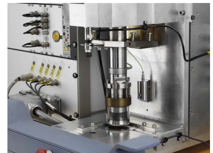
Surface strain sensor for indirect measurement of process forces Load washer
