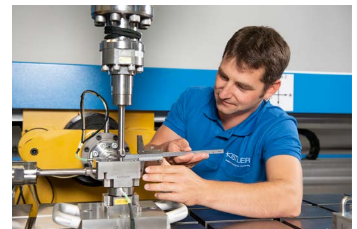
Multi-component force calibration: measuring of cylinder positions
